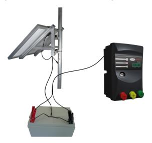
\*\* The Wi-Fi Anywhere® middle lead (load output) will remain unused. The plug pack provided with the energiser will also be unused.
