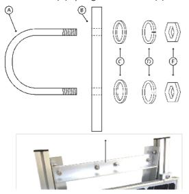
3. Mark the mounting pole. This is where the top of the U-bolt will be. Slide the U-bolts over the pole and tighten when the top bolt aligns with the previous marking.
