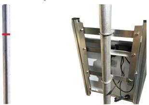
4. Loosen the 6 bolts on the inside of the frame. DO NOT completely remove these bolts. Lift the bottom of the solar panel until the attached arms holding it are angled at 90 degrees. Tighten all 6 bolts again and face the panel north.
