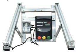
6. If your JVA energiser is fitted, plug it into the middle lead (load output) of the Wi-Fi Anywhere®. The energiser aligator leads and plug pack will be unused (left over).
