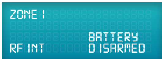
RFI In Battery Fail Alarm
