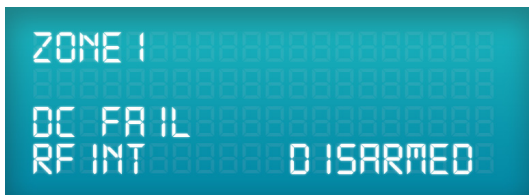
RFI In DC Fail Alarm
