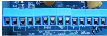
Low Voltage Terminal
